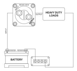
It is important that the negative for this unit is taken from the same battery that the 2 battery switch is isolating. Failure to do this will cause the unit to work erratically. Only one negative must be supplied to each unit for correct operation.
